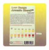
The test is completed with an easy color match.
