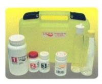
Arsenic Econ Quick Check 481298 300 Tests 12-Minute Test Time Sensitivity / Range: 0,010,025,050,100,250,500,1.000 mg/L
