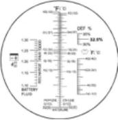
2) Hold daylight plate in the direction of a light source and look into the eyepiece. You will see a circular field with graduations down the center (you may have to locus the eyepiece to see the graduations clearly). The upper portion of the field should be blue, while the lower portion should be white.
