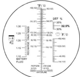
3) While looking into the eyepiece, turn the Calibration Screw until the boundary between the upper blue field and the lower white field meet exactly on 0°C. Once complete, the instrument is calibrated for your current ambient room temperature. When working temperature of the room or environment (not the sample) changes by more than 2C, we recommend recalibrating to maintain accuracy.
