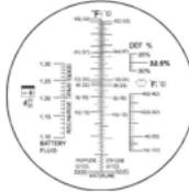
2) Hold daylight plate in the direction of a light source and look into the eyepiece. You will see a circular field with graduations down the center (you may have to focus the eyepiece to clearly see the graduations). The upper portion of the field should be blue, while the lower portion should be white.
