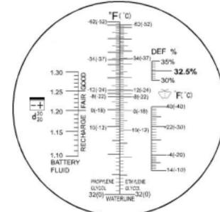
3) Take the reading where the boundary line of blue and white cross the graduated scale. Clean the prism carefully using a damp soft cloth. Do NOT immerse in water. Read warnings below carefully before use.
